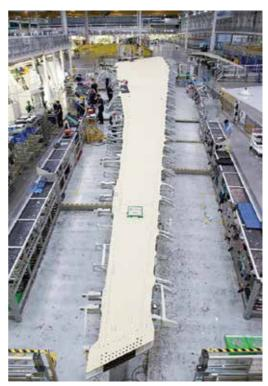
A350 wings being made at Airbus in Broughton.
